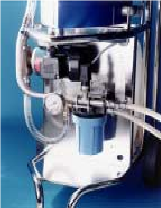
The adjustable backpressure control gives optimal separation efficiency at different working conditions.
