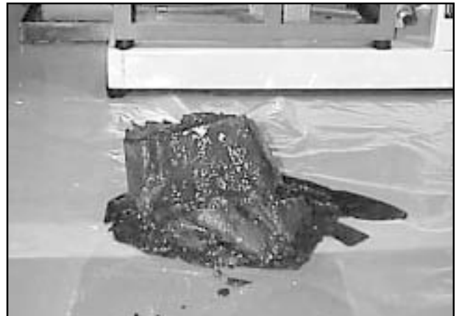
Sludge removed by the Microseparator® centrifuge from a cold header oil tank.
